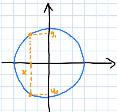
The circle can not be the graph of a function since, if it was the case, the input  $x$  would have two output  $y_1$  and  $y_2$ .
