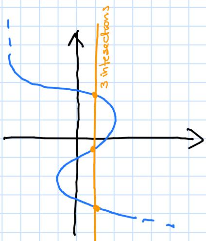
By the vertical line test this is not the graph of a function, since there is a vertical line that has more than one intersection with the curve of the graph
